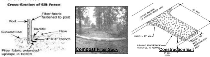
Examples of erosion/sediment controls (Silt Fence and Construction Exit) are available in the BMP manual. Refer to the BMP manual for specifications.
